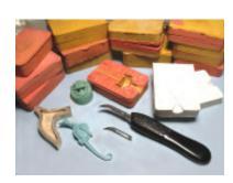
Cutting molds is easier and more precise with a sharp blade. A new Xacto blade is sufficient for cutting RTV molds but is usually not sharp enough for vulcanized rubber. For that it's best to use scalpel blades available from most jewelry supply companies.
