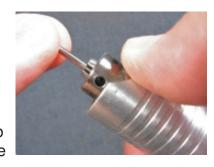
the bur shaft or the drill bit. Then all you have to do is a final tightening with the key.
