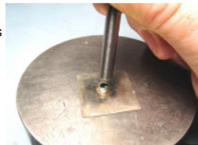
Next you want to force the metal down onto the stone uniformly all the way around. While this can be done by hand, I often gently tap the punch with a hammer. Finally, burnish the bezel by twisting the punch around.
