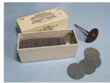
Cutoff wheels are inexpensive and do a great job cutting or shaping steel. You can use them to sharpen tool points, cut piano wire to length, make slots, and sharpen worn drills. Other uses include modifying pliers and making your own design stamps.
