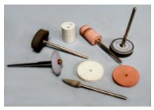
The thicker coin shapes are particularly handy. Cylinder shapes are nice for doing the inside of rings, and knife-edge shapes quickly clean up the solder joint around the outside base of your bezels.
