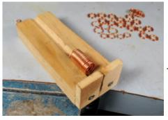
It's about 2 inches wide and 4-5 inches long with a groove cut down its length to cradle the coil of wire and a thin stop attached to the front end.
